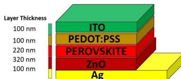
Fig. 16. Simulated Perovskite Solar cell with layer Thickness
